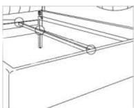
**Step 3.** Attach slat base by inserting 6 screws at each end and middle section. Total 6 x 35mm
