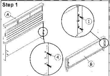
Fix bolt '1' & 4' into position on wood post at headboad & footboard as shown.
