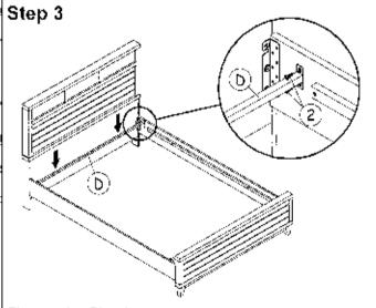
Fix cross bar D to the side rail with bolts '2' as shown.
