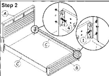
Hook the side rail to the bolt and fix center bolts '1' & '4' as
