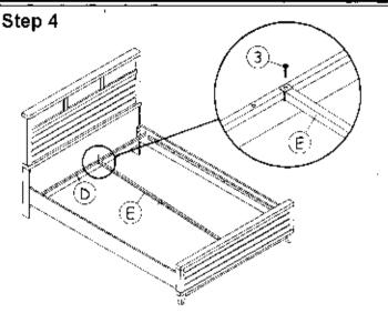
Fix center bar 'E' to the cross bar 'D' with bolt '3' as shown.
