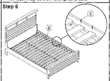
Put wood slats to the side rail support and fix screws [5] at hole as shown.
