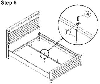
Fix bed support legs as shown and tighten all bolts.
