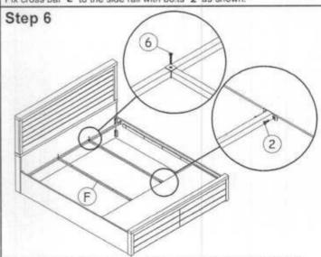
Fix center bar 'F' to the headboard frame and footboard drawer with bolts '2' & '3' as shown
