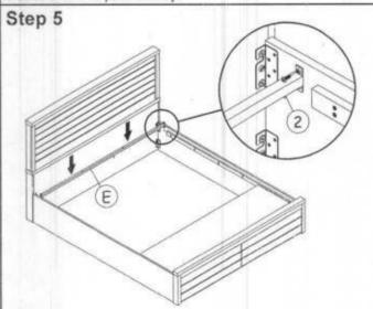
Fix cross bar 'E' to the side rail with bolts '2' as shown.
