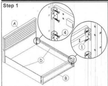
Fix headboard & footboard frame to the side rails with bolts '1' & '4' as shown. Important note: Do not tighten the bolts yet!
