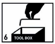
Save the instructions and store the Allen wrench or any supplied tool for later maintenance. After two weeks, check and tighten any loose hardware and repeat again every six months thereafter.
